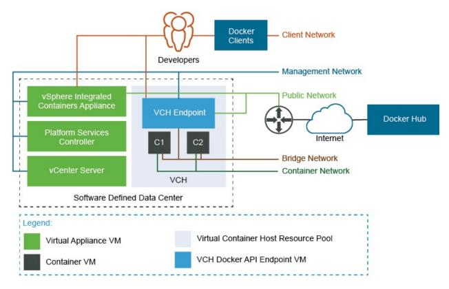
Each VCH requires an IPv4 address on each of the networks that it is connected to. The bridge network is handled internally, but other networks must have a static IP configured on them, or be able to acquire one via DHCP.
